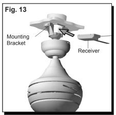
13. Insert the receiver into the mounting bracket with the flat side toward the ceiling (Fig. 13).
